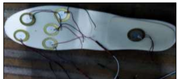
Fig.02 Piezoelectric Sensor Placement on Sole and Modules around the Shoe
